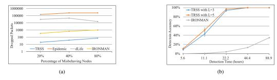
Fig. 7: (a) Dropped packets comparison for TRSS, Epidemic, IRONMAN and dLife with different numbers of misbehaving nodes. (b) Detection Efficiency comparison of TRSS and IRONMAN.
