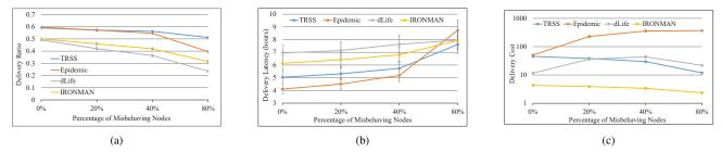
Fig. 6: (a) Delivery ratio comparison of TRSS, Epidemic, IRONMAN and dLife with different numbers of misbehaving nodes. 95% confidence intervals are also presented, showing the variations of all different runs of simulations. (b) Delivery latency comparison of TRSS, Epidemic, IRONMAN and dLife with different numbers of misbehaving nodes. (c) Delivery cost comparison of TRSS, Epidemic, IRONMAN and dLife with different numbers of misbehaving nodes.
