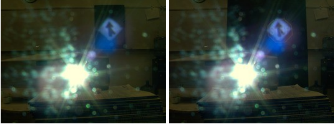
Figure 3.9: Camera-aware attack examples at one meter in perception domain. Left: Creating a Merge sign. Right: Altering a STOP sign (in the background) into a Merge sign.
