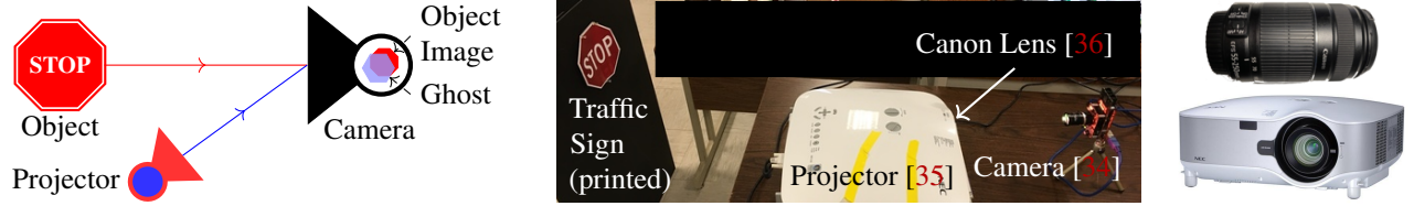
Figure 5: (Left) Attack setup diagram. (Middle) In-lab experiment setup. (Right) Attack equipments: We replaced the original lens of the NEC NP3150 Projector [35] with a Canon EFS 55-250 mm zoom lens [36].
