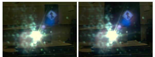
Figure 6: Camera-aware attack examples at one meter in perception domain. Left: Creating a Merge sign. Right: Altering a STOP sign (in the background) into a Merge sign.
